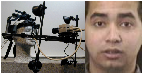
Fig. 4: Mounted-camera device and an example of an input frame
