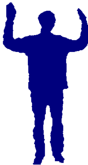
Figure 3.10: Pose required for calibration Kinect for skeleton tracking.
