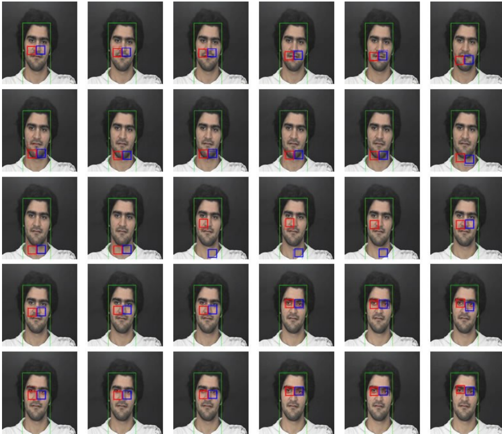
Figure 46: Vertical scanning for a potential eye region.
