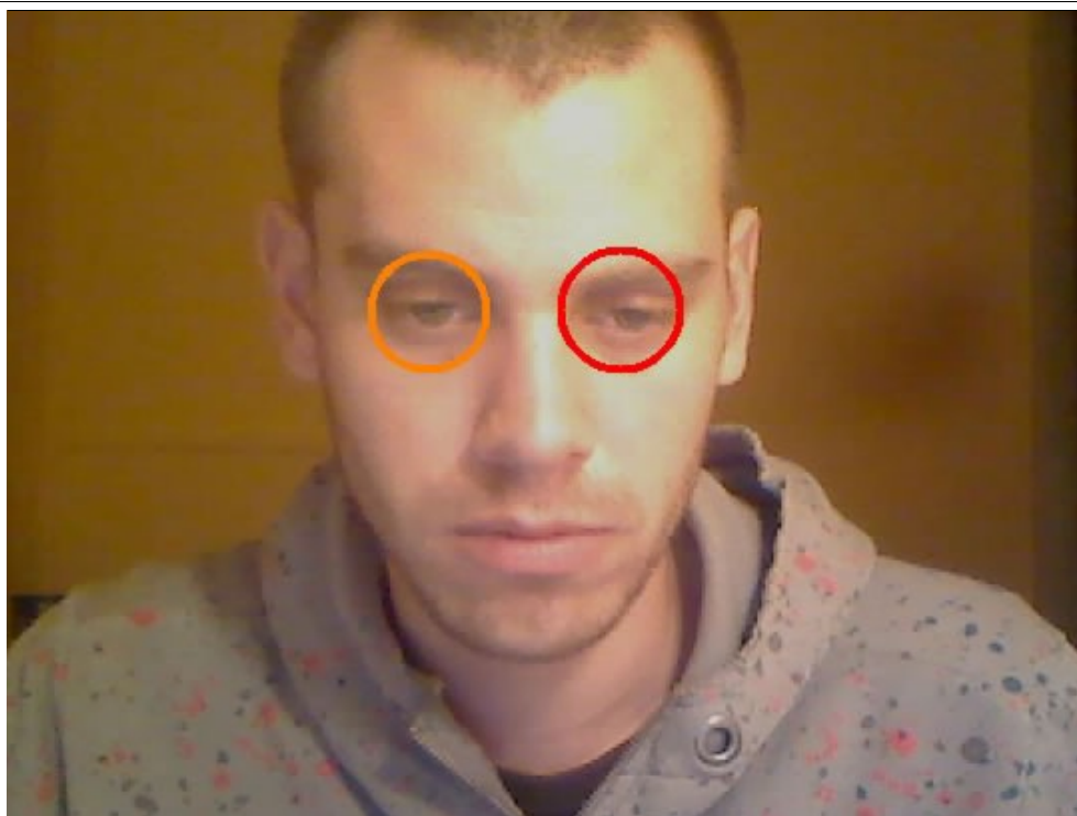
Figure 1: Result of using the standard implementation of the openCV library using haar cascades for detecting the eyes.
