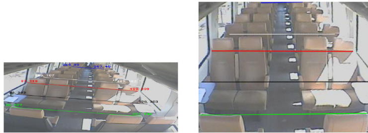
Figure 4.2: Comparison of an original image (left) from the train camera, and the same image after scaling and adjusting (right)
