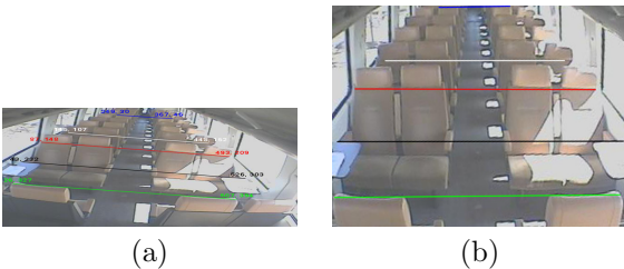
Figure 5: Comparison of an original image from a train camera (a) with the same image after preprocessing (b)
