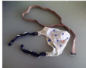
Figure 2.3: Example of a cap for measuring EEG data
