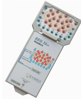
Figure 5.2: Truscan 32 EEG Amplifier
