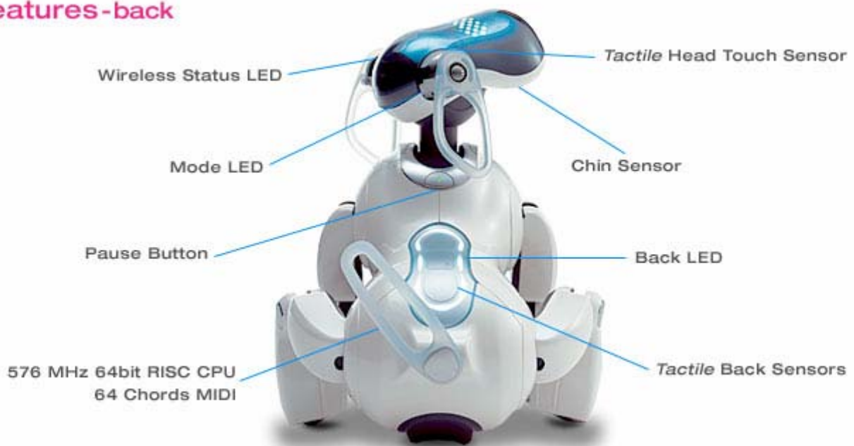
Figure 7: AIBO back features
