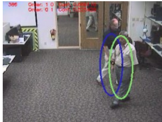
Illustration 2.3: An example of occlusion detection
