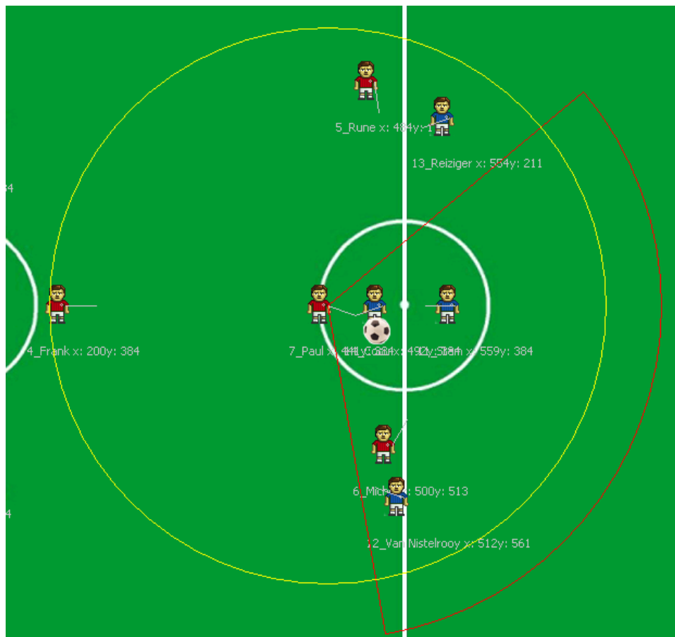
Figure 5.15: The Visual and Aural Sensor Areas of a robot
