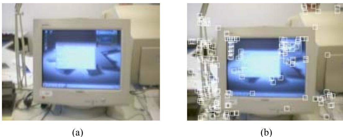
Figure 4.13: A test result example of Sojka corner detection algorithm with noiseGradSizeThresh =14 and corrApparenceThresh =5. (a) Original image. (b) Detection results.
