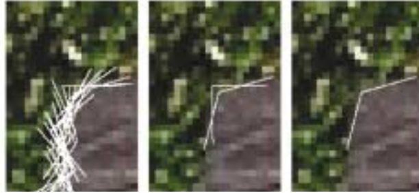
Figure 2.19 Detecting corners from an initial set of candidates, applying an edge model followed by pruning multiple responses if they exist.
