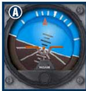
Figure A.6 The Attitude Indicator During the Left Banking
