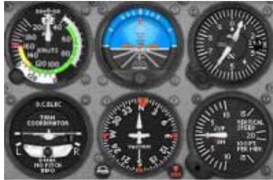
Figure A.5 The 6 Most Important Flight Instruments
