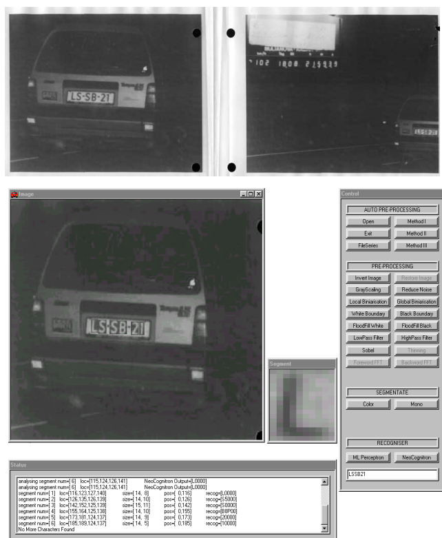
Fig. 6.1 A processing example of a photograph produced by an automated camera operated by the Dutch police. The image cut-out is 320*280 pixels 8-bit grey scaled
