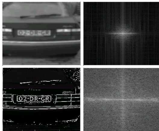
Fig. 1.4 Left the original pictures, right the absolute value of the frequency components. White corresponds to the high values, black to low values
