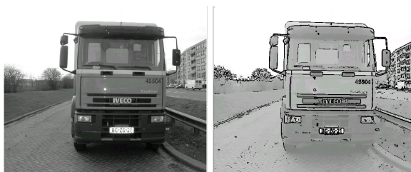
Fig. 1.10a,b Left original image, right the image after the Sobel operation of Equation 1.16 has been applied
