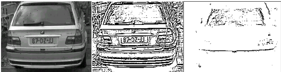
Fig. 6.5 left: 240*190 pixel cutout from original picture #154. middle: binarized image right: no plate left.
