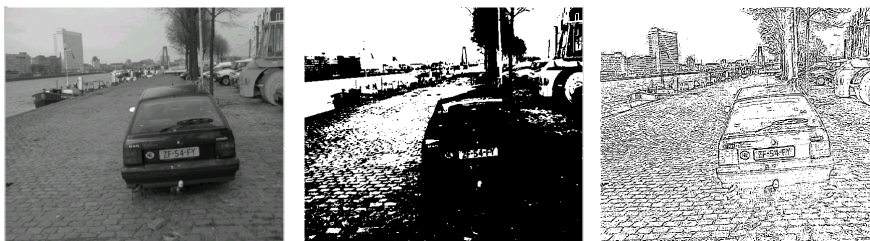
Fig. 1.5a,b,c Left the original picture, global tresholding applied on middle picture, right shows the result of the local tresholding procedure
