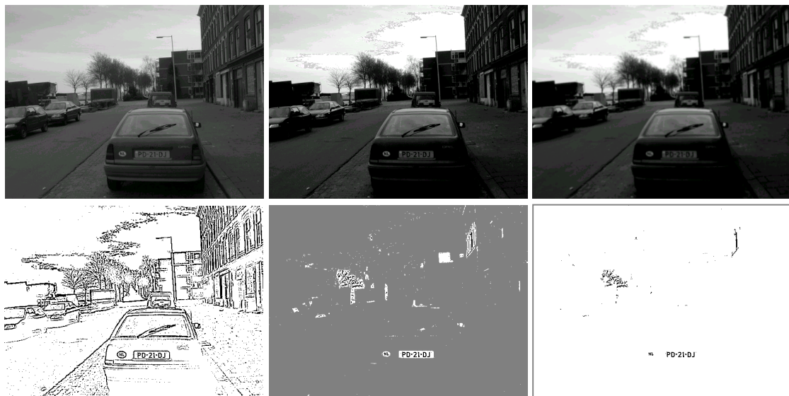
Fig. 9. The image processor steps. Respectively the results of the following image transformations are displayed: original image, grey-scaling, filtering, binarizing and floodfilling twice.
